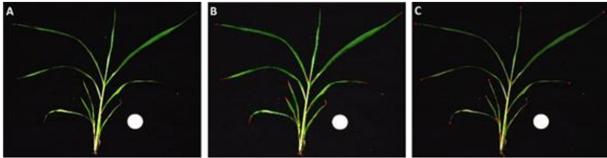
Figure 3 - Example of landmark identification method. Red points represent Raspberry Pi detection of leaf end point. (A) Raw image file used for landmark identification. (B) Acute region detection along contour of plant to flag positions of interest. (C) Reduction to a single informative pixel that can be used for analysis.
