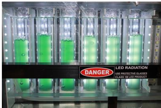
Figure 2 - Growth of cultures in multi-cultivator after switching to air bubbling
