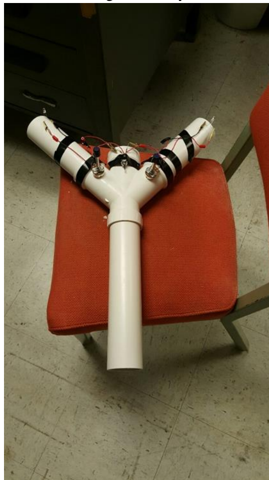
Figure 1 - Y-maze with camera and LED lights. Picture taken by Jimmy Lovett.
