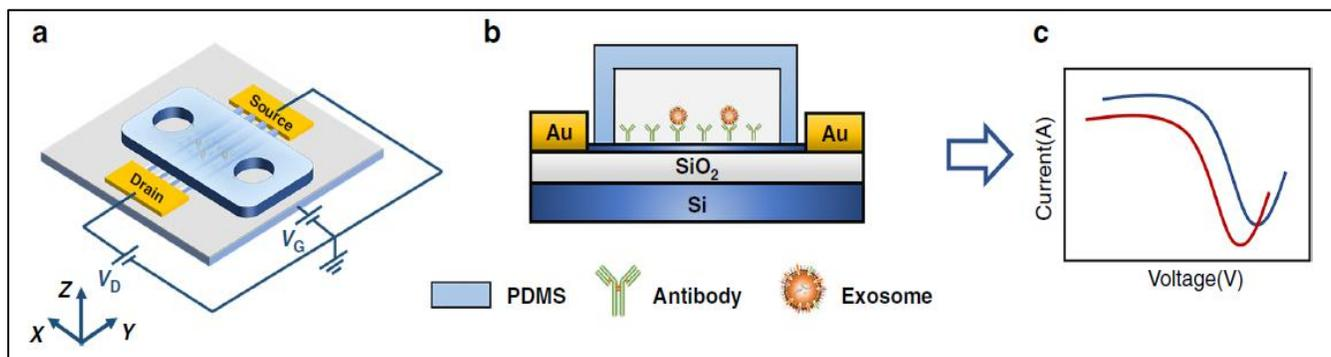
Fig. 2 a Schematic diagram of the Si-NW Bio-FET. b Schematic diagram of the Si-NW Bio-FET cross-section. c Schematic diagram of signal changes [14].
