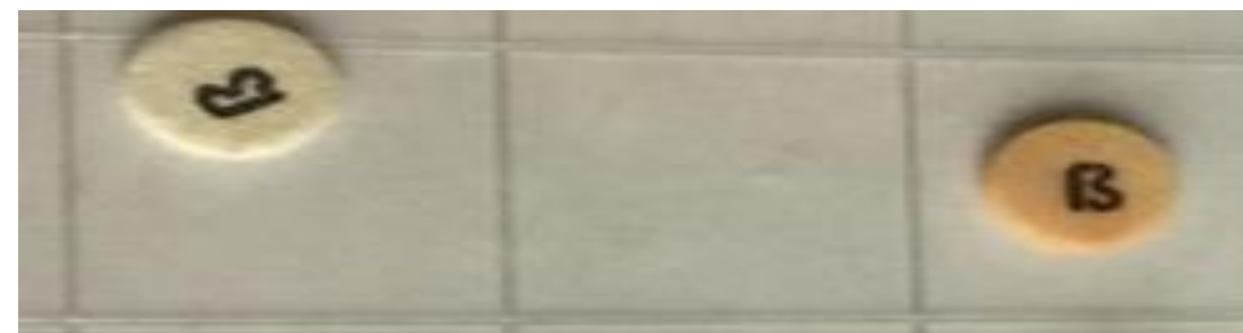
Fig. 2: E. coli was applied to the disk on the right, which exhibited a weak change in color compared to the disk that had nothing applied to it (left).
